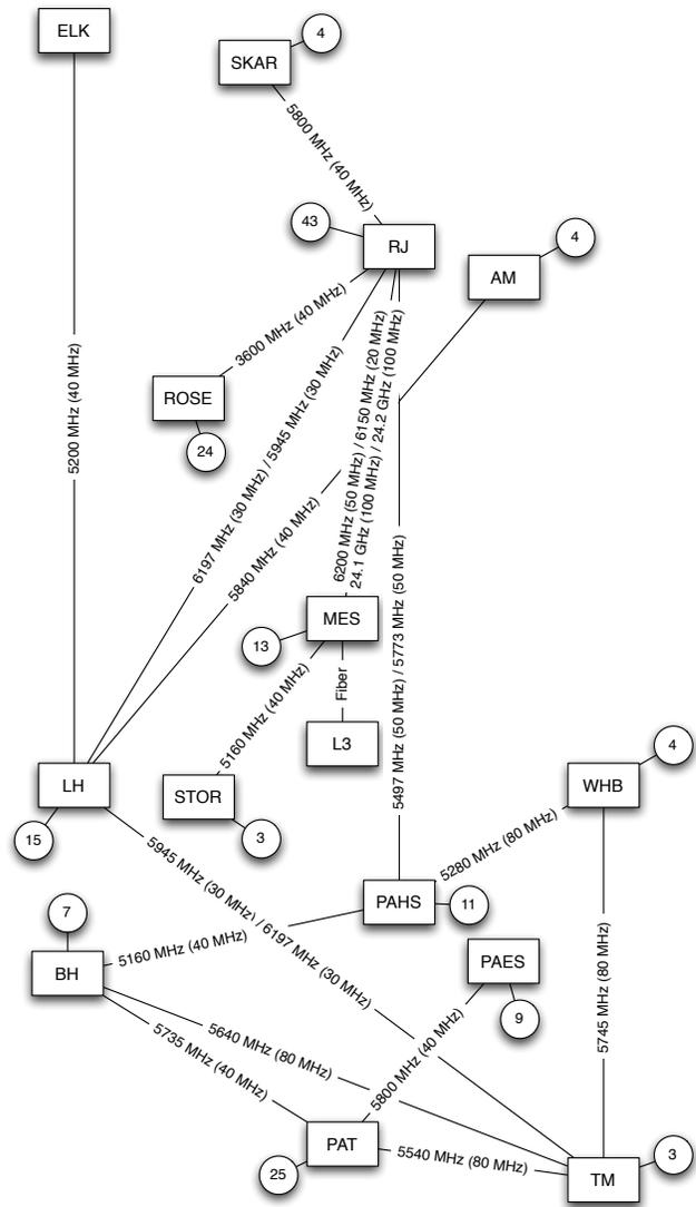
**Figure 2: Our WISP network topology as of Q1 2015. Boxes are major sites, labeled by code names. Circles indicate the number of subscribers connected to those sites at that time. Lines depict backhaul links, with frequency and channel width; for full duplex links, we give TX/RX frequencies from South to North.**
