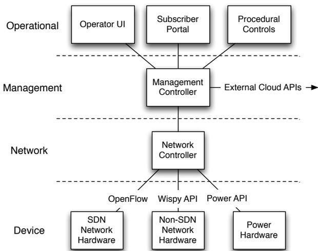
Figure 4: An overview of the subsystems in Celerate.
