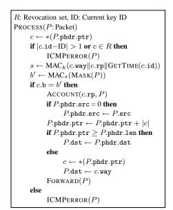
Figure 3: Pseudocode for Platypus forwarding. P is a packet, P.src is the packet's source IP address, and P.phdr is the Platypus header in which src (dst) is the source (destination) address, ptr is the pointer to the current capability and len is the length of the capability list. c is a capability, c.way is the its waypoint field, c.rp is its resource principal field, c.id is its key ID, and c.b is the binding. || denotes concatenation.
