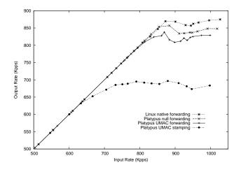
Figure 4: 68-byte packet forwarding/stamping performance.
