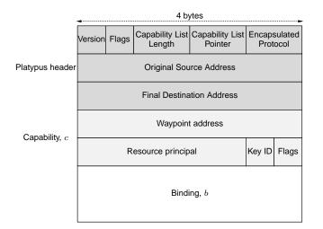
Figure 2: Platypus header format with a single capability and binding attached.
