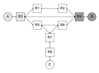
Figure 1: A simple network topology. Hosts A, B, and C all have different ISPs.
