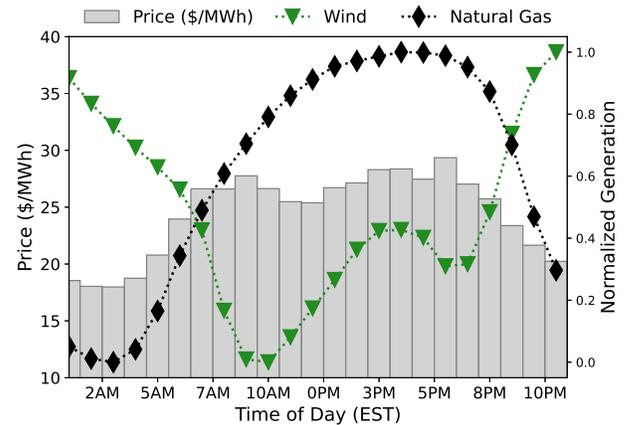
Fig. 1. Gas generation is flexible; wind generation requires wind, and is often out of phase with demand. Prices tend to be lower when wind generation is higher. Based on 2019 price and fuel mix data from MISO [36].
