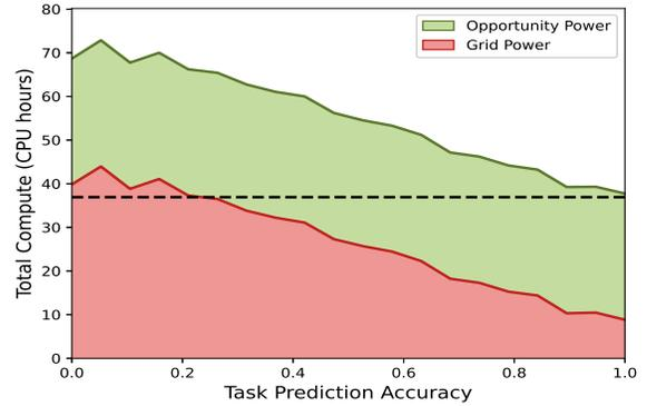
Fig. 5. While more accurate task prediction increases performance, energy can still be saved with relatively low (e.g. 30%) accuracies. Results are shown for machine cycles offloaded in simulation with varied task prediction accuracy and other parameters set based on microbenchmarking results. Simulation ran on MISO price data from 2019.
