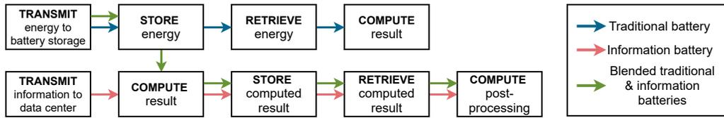
Fig. 2. Energy flows differently through Information Batteries and traditional batteries.
